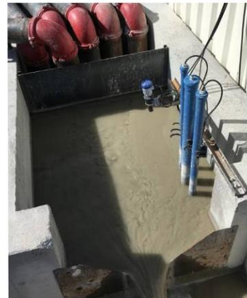
Measurement of pH, turbidity, conductivity and level
