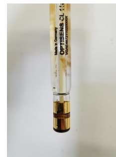
Free chlorine sensor after 8 months of operation
