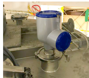
OPTIWAVE 7500 with Tri-Clamp connection
