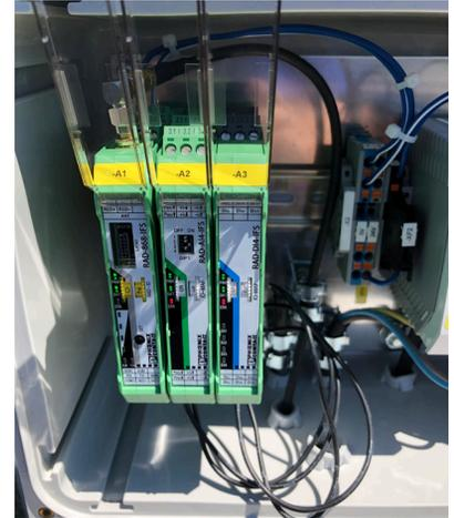
Wireless and I/O modules for the Radioline transmitting unit on the scraper
