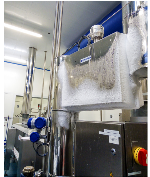
Mass flow measurement of liquid nitrogen for tunnel freezers with the OPTIMASS 6400 F
