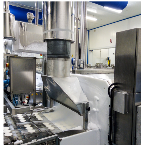
Shock-frozen goat cheese leaving a tunnel freezer; above: OPTIMASS 6400 F
