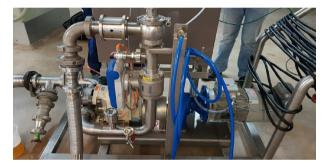
Mobile measuring and control unit with OPTISYS TSS 3050 and OPTIFLUX 6100
