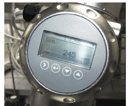
Level measurement of injectable drug products in a mixing tank
