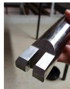
Optical sensor of the OPTISYS SLM 2100
