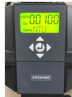
Scattered light measurement according to ISO 7027
