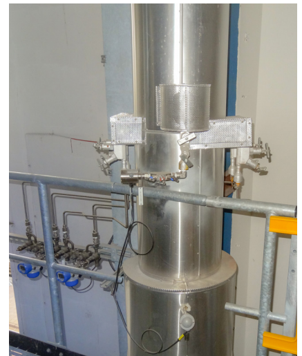
Calibrated meter run with Venturi nozzle, OPTIBAR DP 7060, OPTIBAR PM 3050 and OPTITEMP TRA-S34
