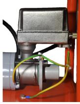
BATCHFLUX 5500 on mobile grout monitoring system
