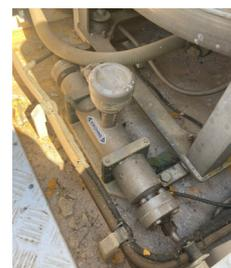
OPTIMASS 7400 F measuring paint for road markings
