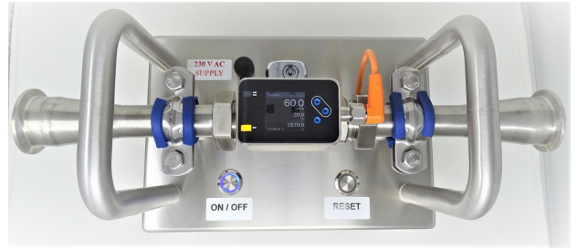
Portable flow system with AF-E 400 mag meter (top view)
