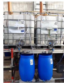
Flow measurement of filtrate water from sludge treatment wetland
