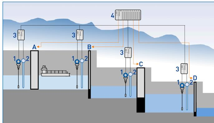
The difference between TDR and hydrostatic level measurements must be <math>< 30 \text{ mm} / 1.18 \text{''}</math>; Deviations between water levels of lock chambers must not exceed a threshold of
