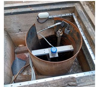
Measurement of water level in a lock chamber
