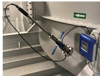
pH measurement in fish silage for acid dosing
