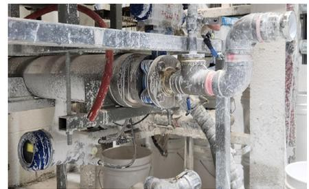
OPTIMASS 7400 for batching of paint additives
