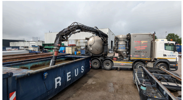
Performance testing of a vacuum excavator using the OPTISONIC 6300 P clamp-on flowmeter
