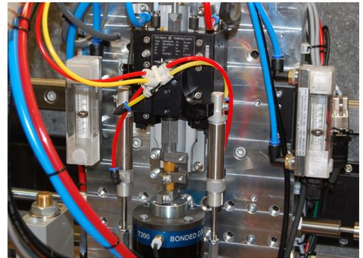
Variable area flow measurement of coolant
