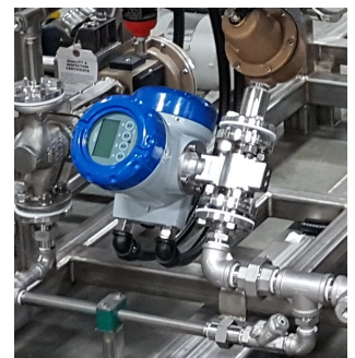
OPTIFLUX 4300 C measuring the flow of emulsifier
