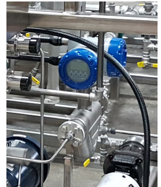
Flow measurement of ASA sizing emulsion with OPTIMASS 6400 C
