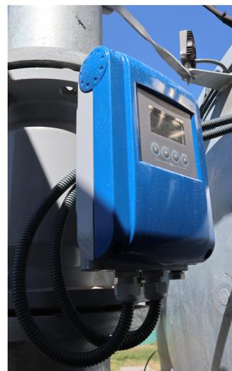
Flow measurement of liquid manure with the OPTIFLUX 2100
