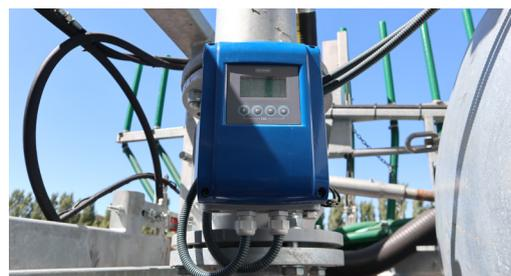
KROHNE flowmeter installed on liquid manure spreader
